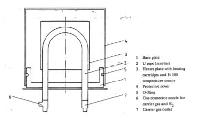
In the ex-version the U pipe is encapsulated and pressure proof. The base plate contains a gas connector and exhaust nozzles for purge gas. The gas connector has a pipe, which extends into the purged shaft behind the installation chamber. This pipe is used to hold the connection lines for heating cartridges and temperature sensor. Purge gas flows from the purged shaft into the methanator housing through this pipe and prevents explosive gas from reaching the heater connections.
